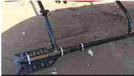
Alpine Aerotech's Bear Paw Kit is compatible with both types of Bell 505 skid gear. Alpine Aerotech Photo
